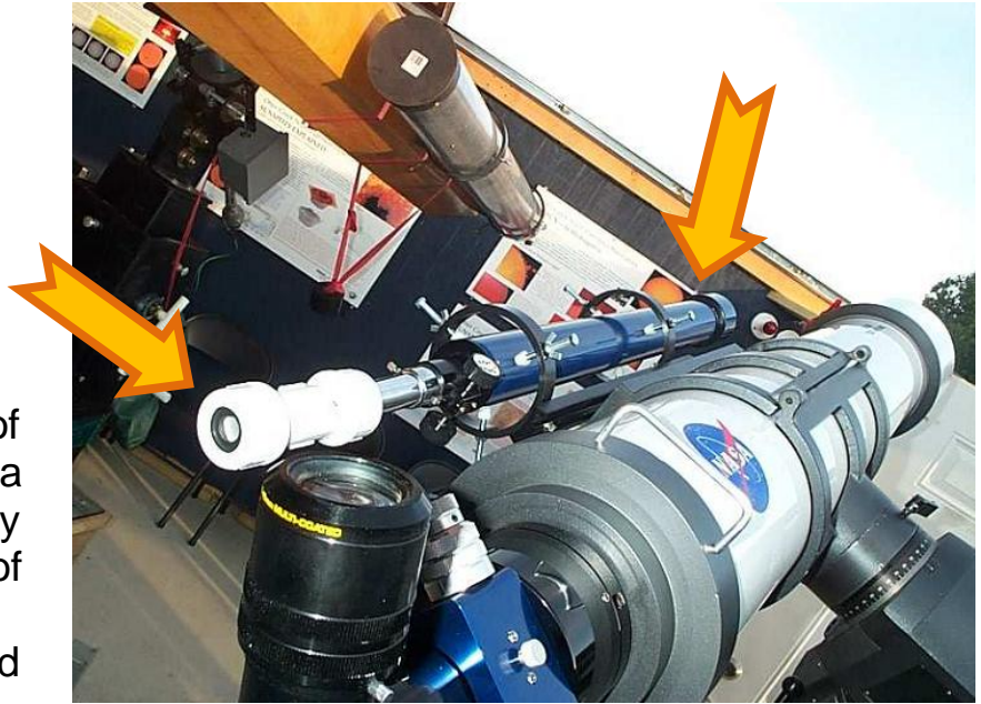
The Galileo telescope at South Harrison, mounted piggy-back on a larger modern refractor. This lets visitors to the observatory make an easy “side-by-side” comparison of what Galileo’s telescope showed him to what modern telescopes reveal to us. The Galileo telescope magnifies 21x.
