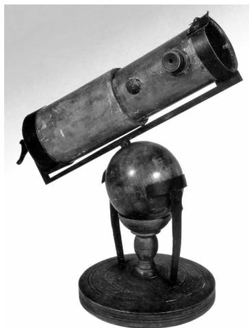
The curve of the mirror in a modern reflector is a parabola -- albeit not as deep as this parabola shown. Isaac Newton, who invented the reflector, actually used a telescope (pictured at left) in which the curve of the mirror was just a segment of a simple circle. However, the parabolic shape produces better images than does the simple circular (or “spherical”) shape. This earliest type of reflector is called a “Newtonian” reflector.
