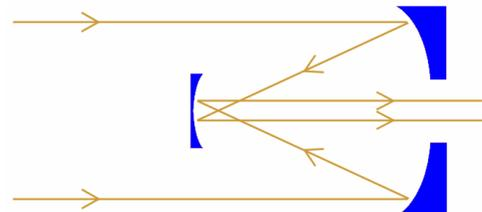
reflected light back through a hole in the primary mirror. The early reflectors caused a stir because their tubes were noticeably shorter than refractors of the same aperture (width) while providing reasonably good images, and shorter telescopes were easier to handle.
