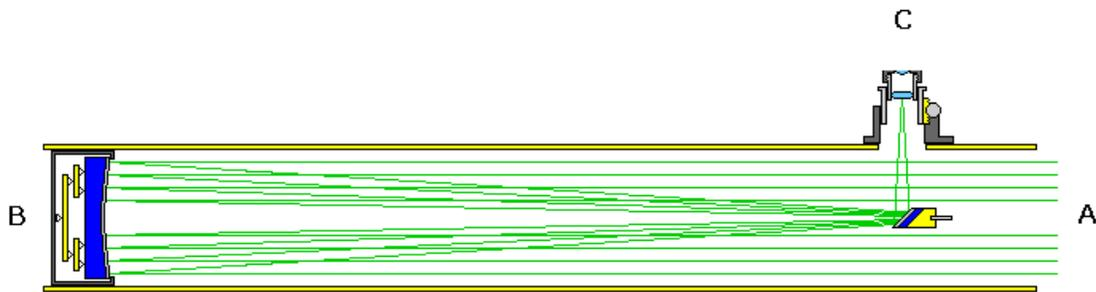
The curve of a reflector’s mirror is similar to the curve of satellite TV dishes. The principle of focusing radiation this way is the same for both. The mathematics and design is fairly simple. In fact, if you have ever taken an algebra course, you probably had to suffer through graphing a parabola like this one.
