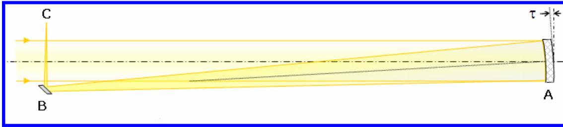
was removed further to the side of the telescope out of the path of the incoming light. This design is the first example of what has become known as “off-axis” reflectors, so-named because such telescopes reflect their light askew with respect to the optical axis of a traditional Newtonian reflector. It is also an “unobstructed” reflector because the light path is not obstructed by the secondary mirror.
